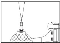
Figure 5. Lubricating the nailer via air inlet.
